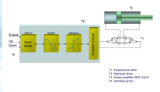
✓ Motor potentiometer function (saving of the last adjusted value and restarting with this value)
