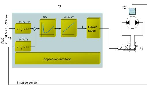
Typical applications: speed control with pulse generators.
