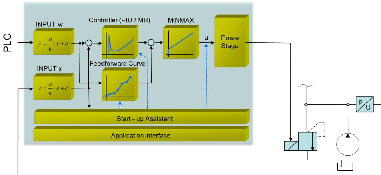
The input signals are first treated with a flexible scaling function.
