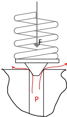
In principle, a pressure relief valve has a very simple structure and has been an indispensable component since the beginning of industrialisation. Of course, the finesse is in the details: tendency to oscillate -> damping, influence of flow forces, tightness, etc.
