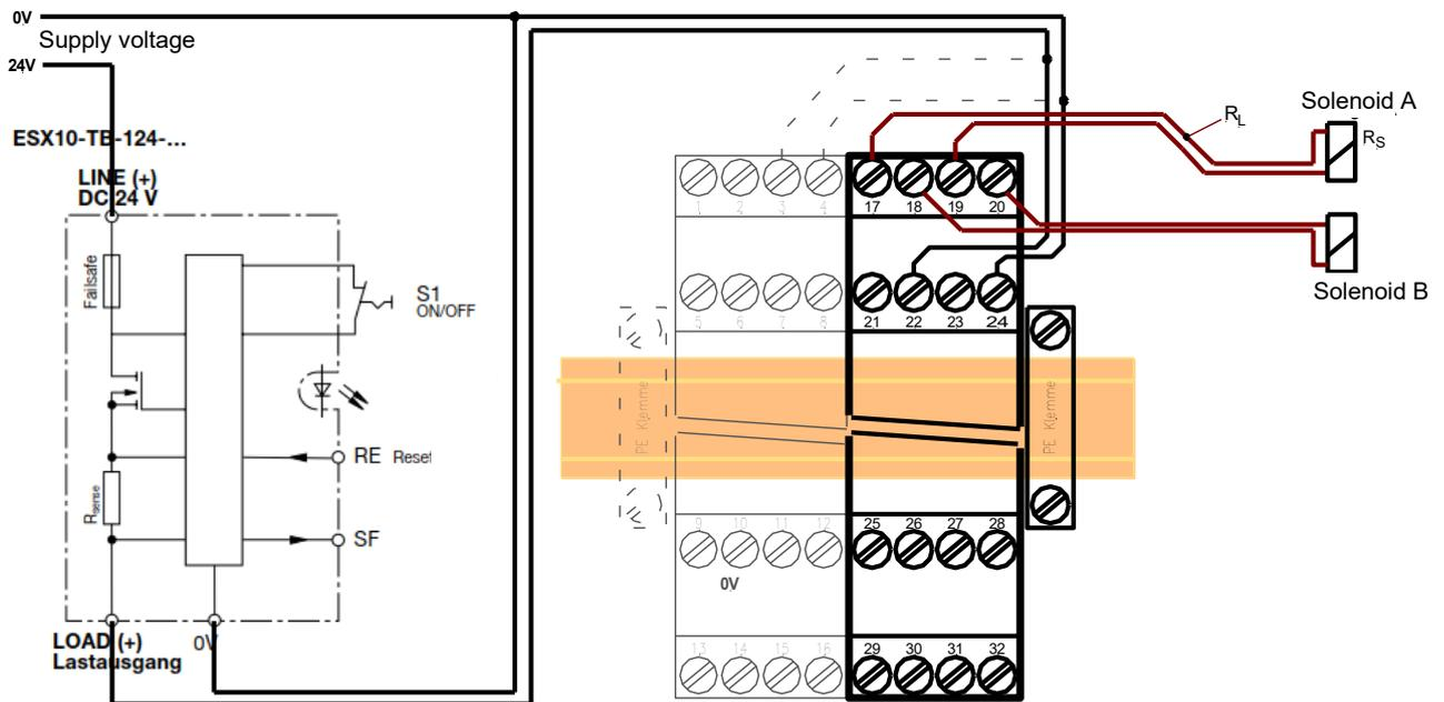
As shown here, the control section of the POS-123-P can also be supplied at terminals 3/4 via the device or can be protected separately.
